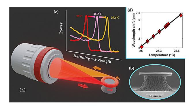
a, An objective lens is used to couple free space light (red beam) into the microtoroid. The resonant scatter light is collected at the opposite edge as indicated by the orange beam. b, Scanning electron micrograph of a microtoroid resonator (SEM image). c, Microtoroid resonance wavelength at different temperatures. d, Resonance wavelength shift vs. temperature. A linear fit is shown as a solid black line. Credit: Sartanee Suebka, Euan McLeod & Judith Su
