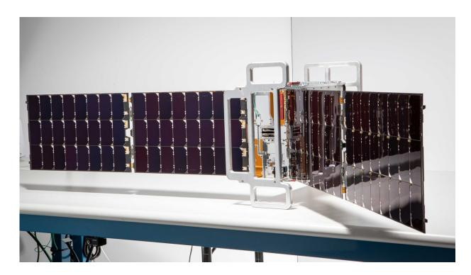
One of the two shoebox-size CubeSats that make up NASA's PREFIRE mission sits on a table at Blue Canyon Technologies. The company built the satellite bus and integrated the JPL-provided thermal infrared spectrometer instrument. Credit: NASA/JPL-Caltech
