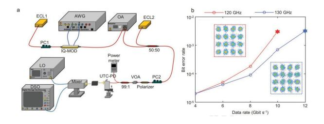
(a) Experimental set-up of the photonic transmission system carrying singlesubchannel 2.5-GHz broadband 16-QAM signals. (b) Relationship between the transmission data rate and the BER achieved in the chip. The insets of (b) show the constellations of transmitted 16-QAM signals below the HD-FEC threshold marked by red and blue stars. Credit: Science China Press
