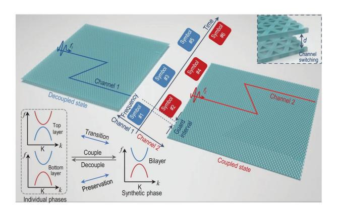
The blue and red rays represent different subchannels over the frequency domain. The subchannel switching is operated at the cost of a temporal guard frame determined by the switching time of interlayer distance *d*. The insets show the simplified diagram of the energy bands with a TP transition mechanism. Credit: Science China Press
