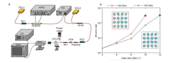
(a) Experimental set-up of the photonic transmission system carrying single-subchannel 2.5-GHz broadband 16-QAM signals. (b) Relationship between the transmission data rate and the BER achieved in the chip. The insets of (b) show the constellations of transmitted 16-QAM signals below the HD-FEC threshold marked by red and blue stars. Credit: Science China Press
