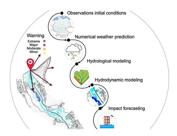
A holistic end-to-end impact-based flood forecasting modeling chain. The state-of-the-art flood early warning system is extended with components of quasi-real-time hydrodynamic and impact forecasting. Observational initial conditions are obtained based on data from ground, radar, satellite, and reanalysis. The Technology Readiness Level (TRL) serves as a scale for evaluating the developmental stage and maturity of a technology. At TRL 1, the technology is
