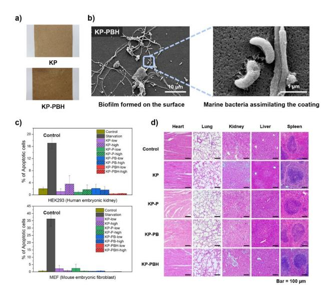
(a) Normal paper and boric acid-crosslinked poly(vinyl alcohol) coated paper,(b) Biodegradation of the coated paper by marine bacteria, (c) Result of cytotoxicity test using human embryonic kidney and mouse embryonic fibroblast cells. (d) Vital organs after one-month exposure of the coated papers to mice.Credit: The Korea Advanced Institute of Science and Technology (KAIST)
