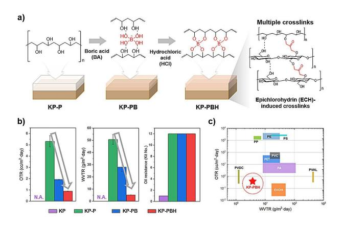
(a) Chemical structure of boric acid-crosslinked poly(vinyl alcohol) coating on paper, (b-c) Oxygen and water vapor barrier properties, (d-f) Tensile strength in dry and moist conditions. OTR: Oxygen transmission rate, WVTR: Water vapor transmission rate. Credit: The Korea Advanced Institute of Science and Technology (KAIST)
