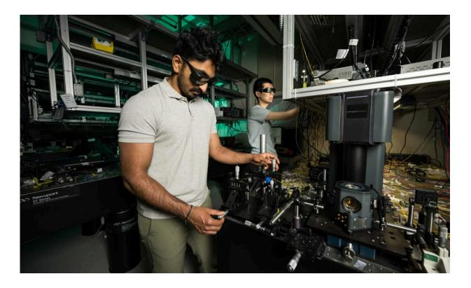
Researchers at the University of Rochester, including optics graduate students Arjun Iyer (foreground) and Wendao Xu, designed acoustic cavities, or tiny echo chambers, to strongly couple surface acoustic waves with light. These devices are simple to fabricate, small in size, and have the ability to handle large amounts of power. Credit: University of Rochester photo / J. Adam Fenster
