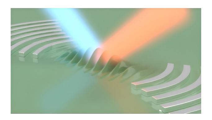
Beams of light, shown in orange and blue, are shined on a surface acoustic wave resonator, where their interactions are controlled by a precisely designed cavity. Inside this echo chamber, the light becomes strongly coupled with the surface acoustic waves. Credit: Arjun Iyer
