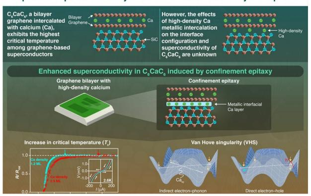
The findings of the study reveal the significance of interfacial interactions for achieving high-temperature superconductivity in composite materials. Credit: Tokyo Tech
