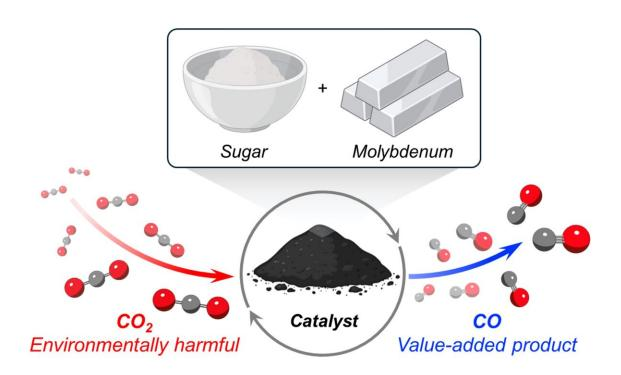
This schematic shows the full process of creating the catalyst and using it to convert carbon dioxide. Credit: Milad Khoshooei
