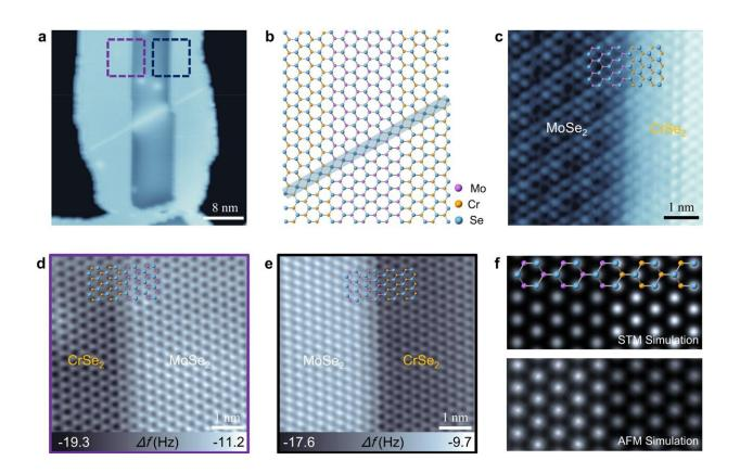
Structural characterization of the MoSe<sub>2</sub>–CrSe<sub>2</sub> lateral heterostructures. Credit: *Nature Communications* (2024). DOI: 10.1038/s41467-024-46087-0
