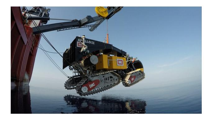
Deployment of Royal IHC's Apollo II pre-prototype nodule collector vehicle from the aft of RV Sarmiento de Gamboa during the 2018 field test in Málaga Bight. Credit: Alberto Serrano.
