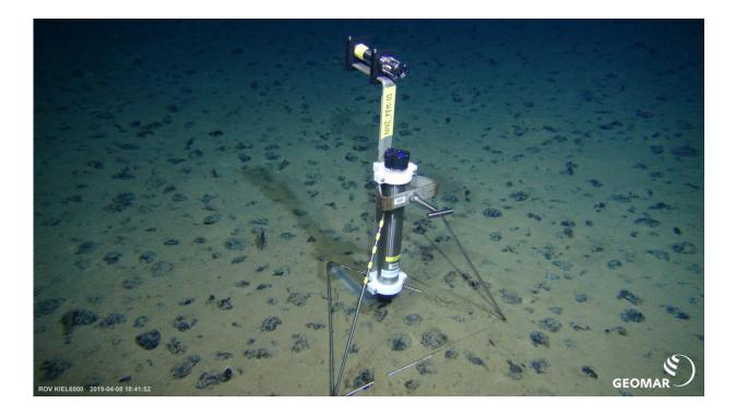
Sensor frame deployed among the polymetallic nodules in the Clarion-Clipperton Zone in the NE equatorial Pacific Ocean. The top sensor is a turbidity sensor recording suspended particulate matter loads and the bottom vertically mounted sensor is an ADCP (Acoustic Doppler Current Profiler) used for recording current speed and direction, as well as vertical profiles of turbidity. Credit: ROV KIEL 6000 (GEOMAR, Kiel).
