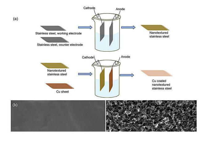
a) Nanotextured stainless steel fabrication and its modification using Cu by electrochemical techniques. b,c) SEM and d,e) AFM, b,d) images of pristine
