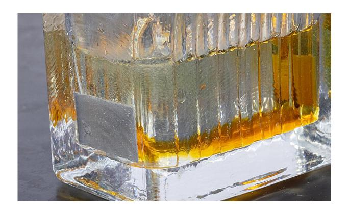
During the Tripathi's electrochemical process, current and an acid electrolyte etch nano-sized needle-like structures on the surface of stainless steel. The structures are able to destroy bacterial cells. Credit: *Small* (2024). DOI: 10.1002/smll.202311546
