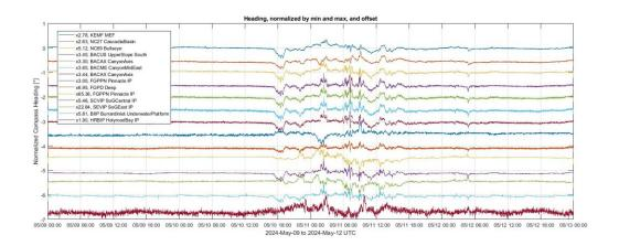
Compass data captured by ONC's major cabled subsea observatories VENUS and NEPTUNE off Vancouver Island, at Burrard Inlet on the Pacific Coast, and at Conception Bay on the Atlantic coast shows the magnetic field distortion occurring during a solar storm from May 10–12 (UTC), 2024. Credit: Ocean Networks Canada
