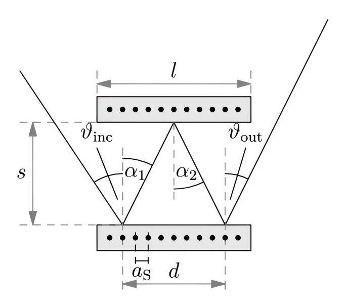
The team's setup consists of two parallel nano-structured slabs that reflect an incident matter beam three times. Credit: *The European Physical Journal D* (2024). DOI: 10.1140/epjd/s10053-024-00829-3
