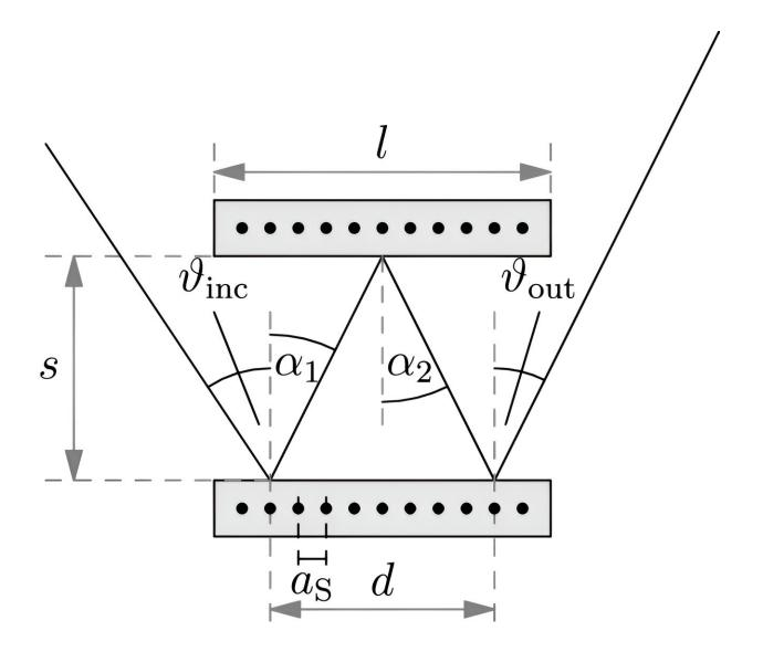
The team's setup consists of two parallel nano-structured slabs that reflect an incident matter beam three times. Credit: *The European Physical Journal D* (2024). DOI: 10.1140/epjd/s10053-024-00829-3
