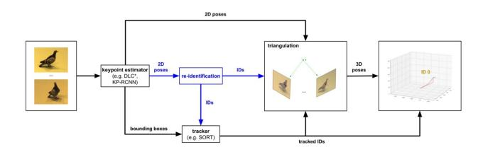
3D-MuPPET. The framework consists of a pose estimation and tracking module, into which we can readily slot any state of the art pose estimator and tracking method. We identify all individuals in all views (blue part) in the first frame only. In the subsequent frames we track the identities with SORT. 3D-MuPPET predicts 3D poses together with IDs from multi-view image input using triangulation. Credit: *International Journal of Computer Vision* (2024). DOI: 10.1007/s11263-024-02074-y
