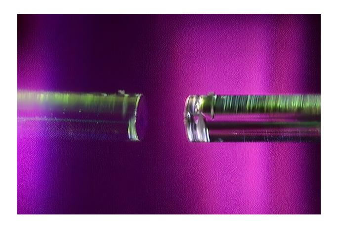
The heart of this study is a fiber microcavity. Here, one can see a small concave depression in the surface of an optical fiber. The researchers used a microcavity with two concave mirrors, but this image of a single concave microcavity makes it easier to see the fiber mirror setup. Photo by Carlos Saavedra/UW–Madison
