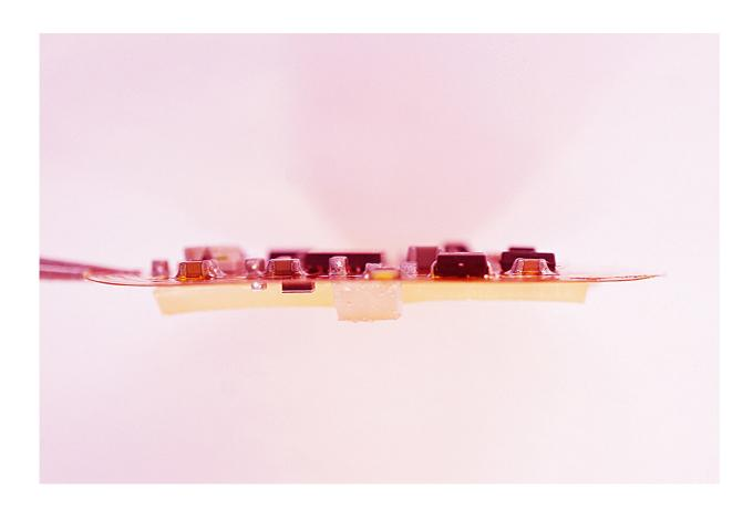
A wafer-thin patch incorporates a flexible electronic circuit, a gel made from tapioca starch and gelatin, and friendly bacteria that help treat skin conditions. Credit: Jiuyun Shi and Bozhi Tian/University of Chicago
