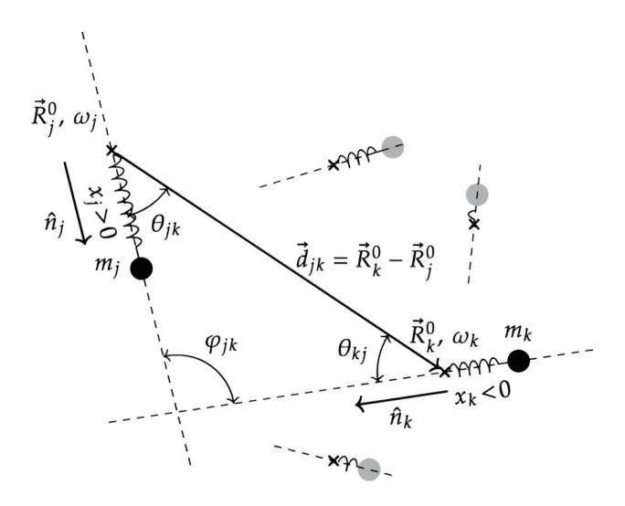
A system of one-dimensional quantum harmonic oscillators. The various angles are defined in Eq. (60). Note that for the most general three-dimensional arrangement the two dashed lines will not intersect. Credit: *Physical Review X* (2024). DOI: 10.1103/PhysRevX.14.021022
