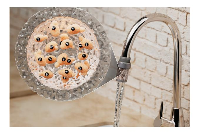
Engineered yeast-containing hydrogel capsules could be used to remove lead from contaminated water rapidly and inexpensively. The work, from MIT and Georgia Tech researchers, could be especially useful in low-income areas with high lead contamination. Credit: MIT
