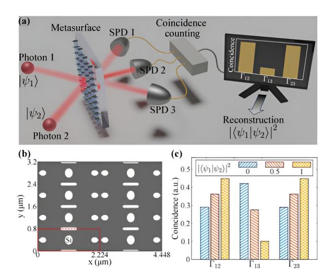
a) Schematic of the metasurface-enabled single-shot characterization of twophoton indistinguishability. Credit: *Optica* (2024). DOI: 10.1364/OPTICA.516064
