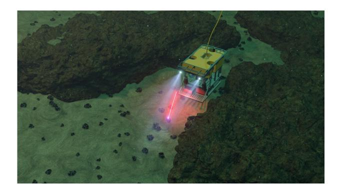
Illustration of a diving robot that uses laser-induced plasma spectroscopy (LIBS) to analyse materials in the deep sea in an environmentally friendly way. Credit: INP
