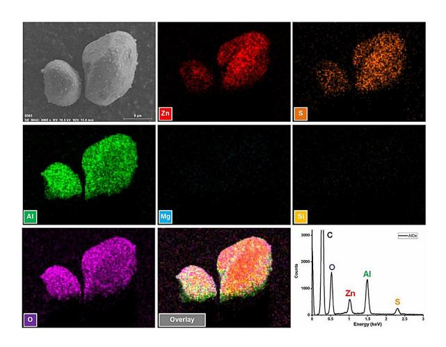
Composition analysis (SEM, elemental mapping images, and EDS spectrum) of commercial ZnS:Cu microparticles exhibiting bright friction-induced luminescence with PDMS. Credit: *Small* (2024). DOI: 10.1002/smll.202307089
