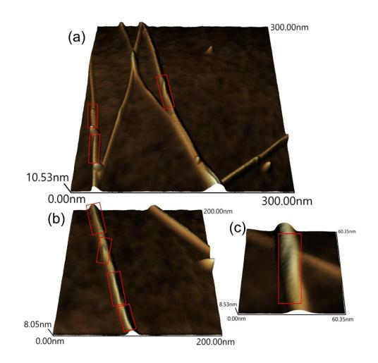
Topographic images of surfactant molecules (indicated by red rectangles) on CNT bundles observed by Frequency-Modulated Atomic Force Microscopy (FM-AFM). Instead of the wet spinning, where the dispersion is injected in methanol, the CNT was spin-coated with diluted dispersion on a hydrophilic  $SiO_2/Si$ substrate and rinsed with methanol. Credit: Masakazu Nakamura
