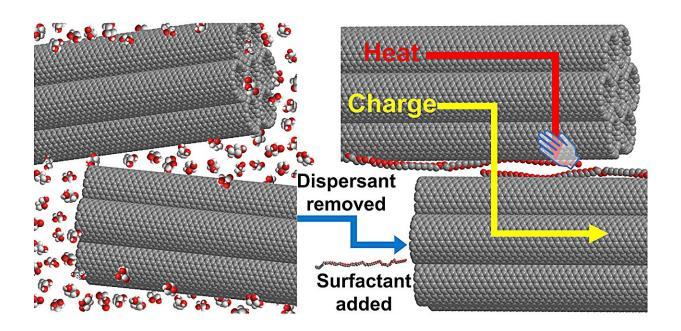
The novel method proposed by researchers for dispersing carbon nanotubes (CNTs) uses glycerol as a dispersant and polyoxyethylene(50) stearyl ether as a surfactant. This method aligned the carbon nanotubes and embedded surfactants between CNT bundles, enhancing electrical conductivity while suppressing thermal conductivity, resulting in significant improvements in the thermoelectric performance of CNTs compared to conventional methods. Credit: Masakazu Nakamura
