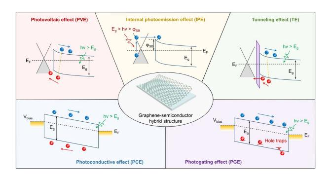
As a representative two-dimensional material, graphene possesses unique optical and electrical properties that hold immense promise in various fields, particularly in photodetection. Nonetheless, its atomic-level thickness results in weak light absorption, seriously limiting the enhancement of key performance indicators for graphene photodetectors. Credit: Advanced Devices & Instrumentation
