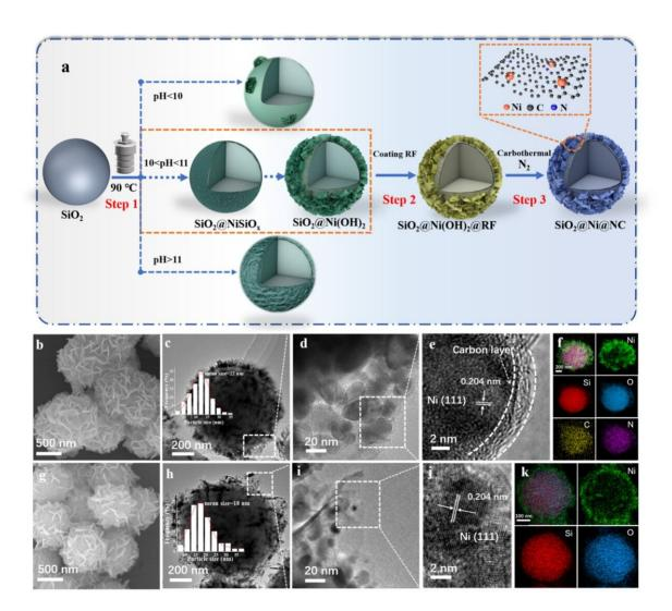
(a) Schematic illustration of the synthesis procedure for SiO<sub>2</sub>@Ni@NC; the corresponding characterization images (b–f) of SiO<sub>2</sub>@Ni@NC and (g–k)
