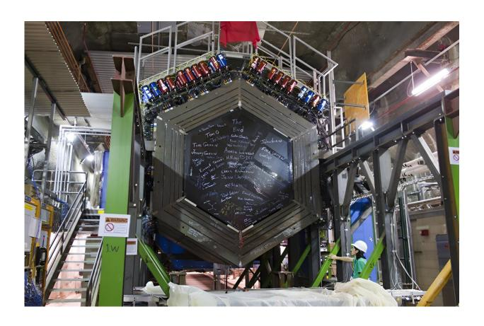
The particle detector used in the MINERvA experiment enabled scientists at DOE's Fermilab to use neutrinos to measure the size and structure of protons. Credit: Fermilab
