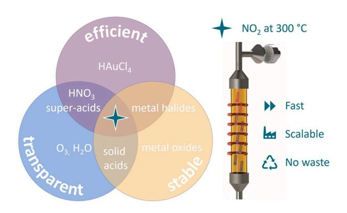
Comparison of various doping agents for making carbon nanotubes more efficient (electrically conductive), transparent, and stable. The Skoltech study demonstrates that nitrogen dioxide (NO<sub>2</sub>) treatment at 300 degrees Celsius — a fast, scalable, and wasteless technology — combines the best of all worlds. The resulting films could enhance renewable energy generation and the performance of gadgets. Credit: Eldar Khabushev et al.
