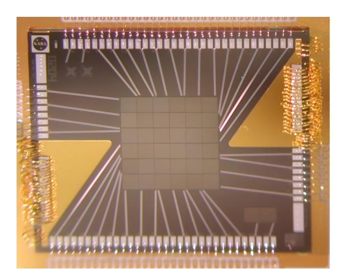
The square structure at the center of this image shows the 6-by-6-pixel microcalorimeter array at the heart of Resolve, an instrument on XRISM (X-ray Imaging and Spectroscopy Mission). The array measures 0.2 inches (5 millimeters) on a side. The device produces a spectrum of X-ray sources between 400 and 12,000 electron volts—up to 5,000 times the energy of visible
