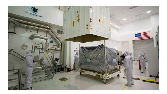
At JPL on May 17, members of the Roman Coronagraph Instrument team use a crane to lift the top portion of the shipping container in which the instrument was stored for its journey to NASA's Goddard Space Flight Center. Credit: NASA/JPL-Caltech
