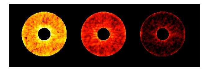
This graphic shows a test of the Roman Coronagraph Instrument that engineers call "digging the dark hole." At left, starlight leaks into the field of view when only fixed components are used. The middle and right images show more starlight being removed as the instrument's moveable components are engaged. Credit: NASA/JPL-Caltech
