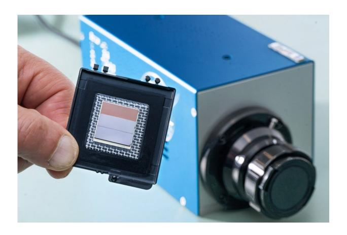
Goddard engineer Murzy Jhabvala holds the heart of his Compact Thermal Imager camera technology – a high-resolution, high-spectral range infrared sensor suitable for small satellites and missions to other solar-system objects. Credit: NASA
