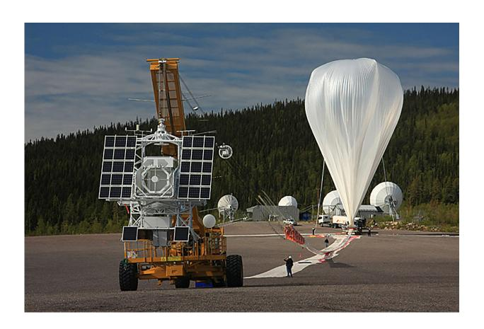
Technicians attach the SUNRISE payload to its balloon and parachute from the launch site in Kiruna, Sweden, during the 2009 campaign. The mission returns for the 2024 Sweden Long-Duration Scientific Balloon Campaign as one of four primary missions set to launch between May and July. Credit: University Corporation for Atmospheric Research
