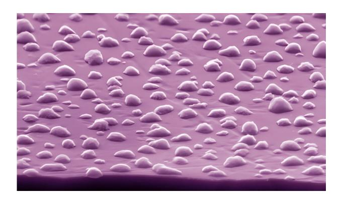
Scanning Electron Microscope (SEM) image of the copper dewetted nanoparticles with antimicrobial properties over the glass substrate. Credit: ICFO
