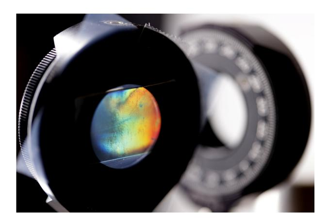
This composite film can twist light into a spiral, thanks to microscopic grooves that cause horizontally and vertically oscillating light waves to pass through the film out of phase. Unlike existing materials that can do this, the film maintains its light-twisting properties when heated up to 250 degrees Celsius. Credit: Brenda Ahearn, Michigan Engineering.
