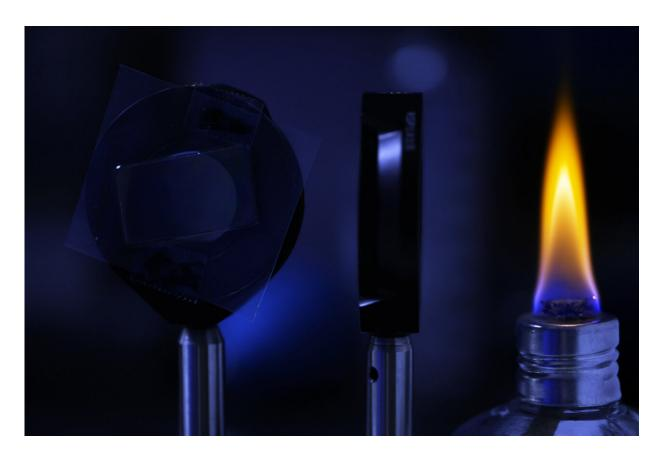
To measure how well the film twists light at high temperatures, U-M researchers use a small flame as a light and heat source. Credit: Brenda Ahearn, Michigan Engineering.
