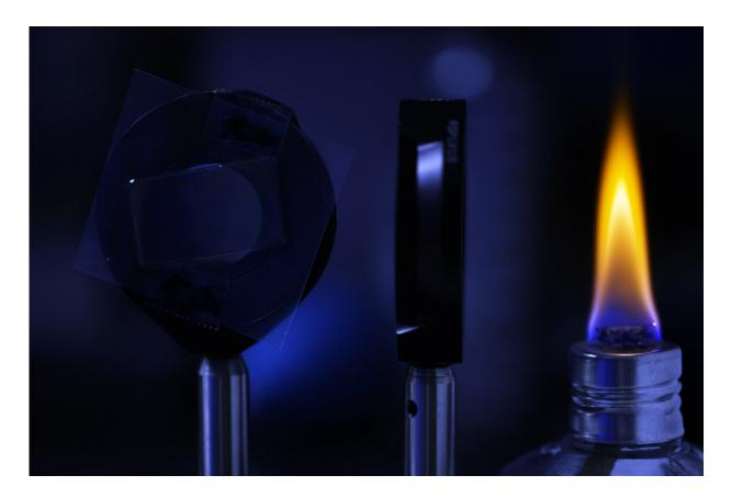
To measure how well the film twists light at high temperatures, U-M researchers use a small flame as a light and heat source. Credit: Brenda Ahearn, Michigan Engineering.
