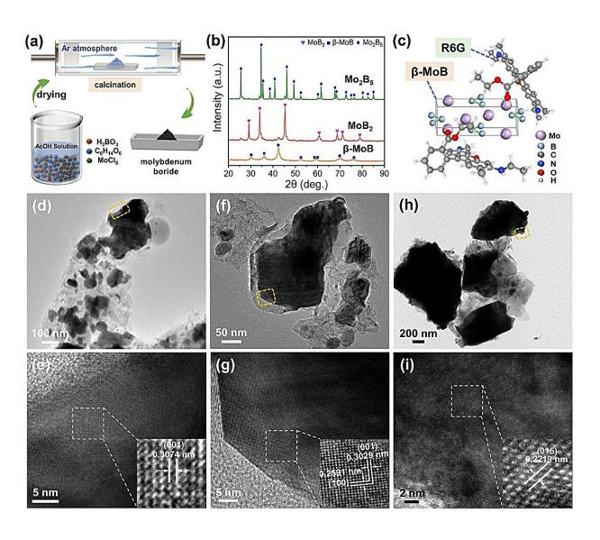
Preparation process and microstructure of molybdenum boride ceramics. Credit: Hu Mengen
