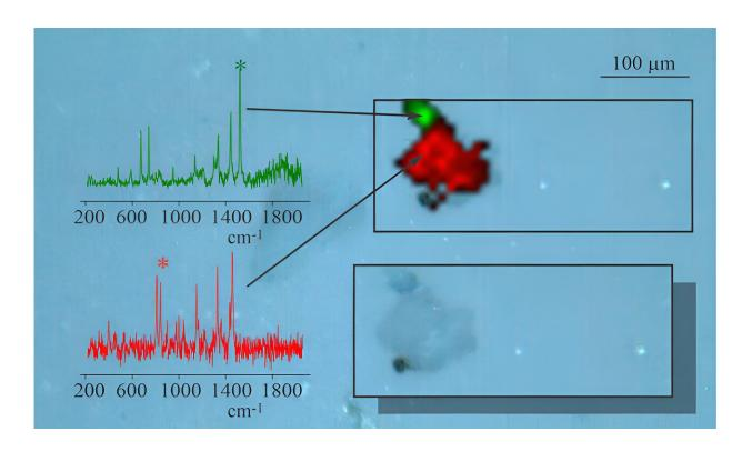
This image, generated in a lab and based on the Raman spectra, shows a microplastic particle within a 100 micrometer area. The false-color images of green and red match for specific polymers detected in the particle. Credit: Luis Medina Faull
