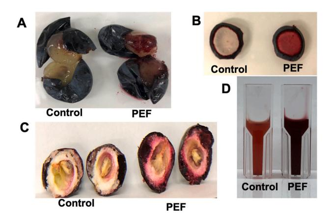
Visual observation of control and PEF (0.85 kV/cm, 300 pulses) treated Concord grape berries after crushing (A), fresh sample cross section (B), freeze dried sample center cross section (C) and grape juice (D). Credit: *LWT* (2024). DOI: 10.1016/j.lwt.2024.116002
