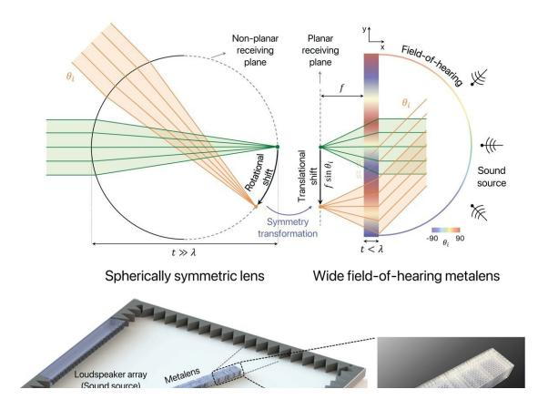
Conceptual illustration demonstrating the realization of a wide field-of-hearing metalens via symmetry conversion of a spherically symmetric Lunberg lens. Credit: POSTECH
