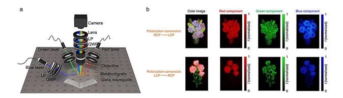
(a) Schematic diagram of the experimental system for full-color imaging. (b) Experimental results of the waveguide-based full-color metahologram. Two crosstalk-free full-color holographic images ("lilac" and "rose") are selectively projected when the metahologram is illuminated simultaneously by red, green, and blue guided incident lights all having right circular polarization or left
