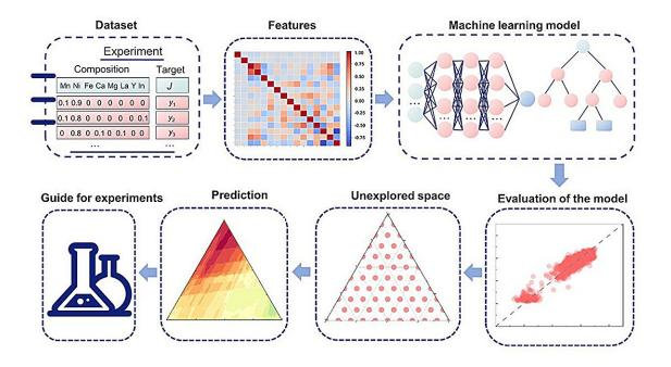
Workflow of the ML-based analytical process employed to explore multicomponent ORR catalysts under alkaline conditions. Credit: *Journal of Materials Chemistry A* (2024). DOI: 10.1039/D4TA01884B
