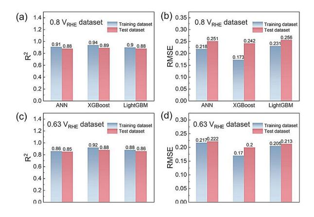
(a–b) Comparison of (a)  $R^2$  and (b) RMSE among the models built by ANN, XGBoost, and LightGBM on the training and test sets. (c–d) Comparison between the experimental and predicted values by XGBoost on the (c) training and (d) test sets. The unit of RMSE is  $lg(\mu A \cdot cm^{-2})$ . Credit: *Journal of Materials Chemistry A* (2024). DOI: 10.1039/D4TA01884B
