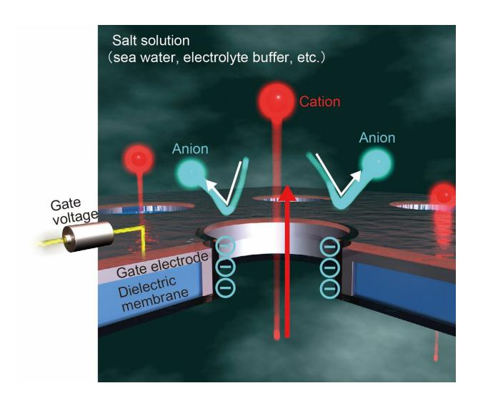
Schematic illustration depicting gate voltage control of ion selectivity in a nanopore. Credit: Makusu Tsutsui
