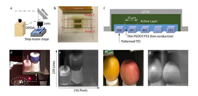
The schematic illustrations and performance of a SWIR image system based on linear image arrays using organic photodiodes reported in this work. Credit: *Chinese Journal of Polymer Science*
