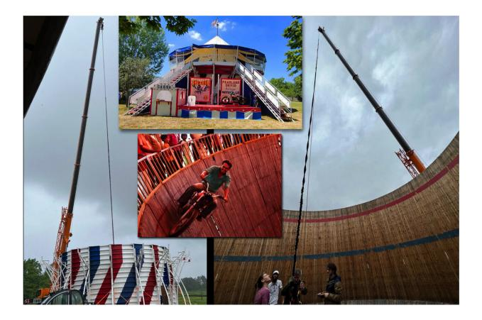
Top inset shows the Wall of Death (WoD) used in this investigation; left picture represents its 'naked' version, with the cap removed as to allow the telescopic crane to hang the body weight unloading bungee cords from a height of 36 m; right picture shows the vertical wall inside the WoD where horizontal running experiments took place at emulated (vertical) lunar gravity; middle inset displays
