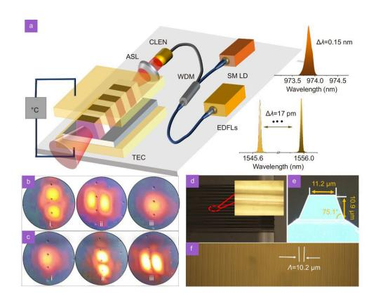
a) Schematic of the temperature/wavelength-dependent spatial mode steerable SFG device; (b) in the temperature steering scheme, the detected up-conversion lights with (i) TM01, (ii) TM10, and (iii) TM00 modes at 30°C, 40°C, and 60°C, respectively, on a white broad; (c) in the wavelength steering scheme, the
