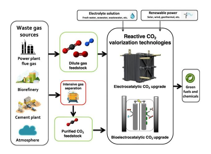
Overview of emerging  $CO_2$  capture and conversion pathways. Proposed process flow for electrified  $CO_2$  conversion with selection of waste gas feedstock, omission or inclusion of gas separation device, and choice of  $CO_2$  conversion nanotechnology. Credit: *Environmental Science: Nano* (2024). DOI: 10.1039/D3EN00912B
