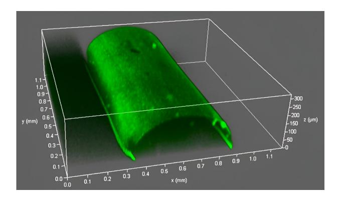
3D image of a VasFluidic channel (laser confocal scanning microscope image). Credit: *Nature Communications* (2024). DOI: 10.1038/s41467-024-45781-3
