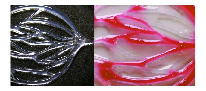
A VasFluidic system with multi-branch channels, and the channels perfused with liquid inside. Credit: *Nature Communications* (2024). DOI: 10.1038/s41467-024-45781-3
