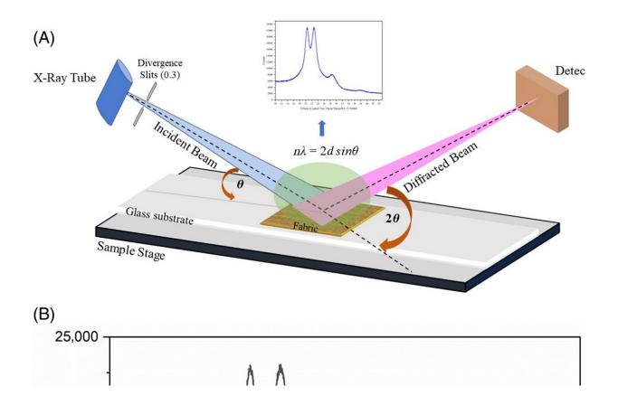
(A) Schematic diagram of performing XRD on fabric specimen. (B) The X-ray diffractogram shows the amorphous and crystalline region of a para-aramid/PBI fiber blended fabric (Fabric MA). Credit: *Journal of Polymer Science* (2024). DOI: 10.1002/pol.20230950
