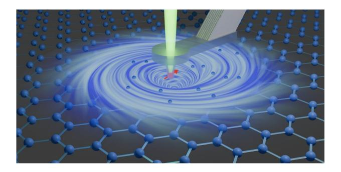
Using a magnetic field sensor (red arrow) inside a diamond needle, researchers at ETH imaged electron vortices in a graphene layer (blue). Credit: Chaoxin Ding
