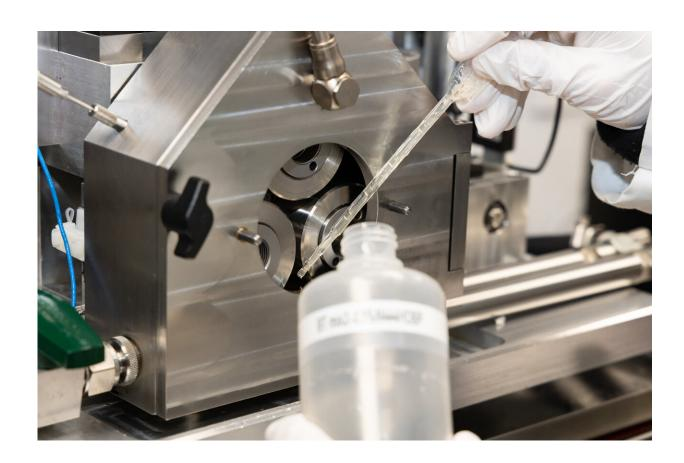
Testing with ORNL tribology equipment found that new ionic liquid-based lubricant additives developed for water turbines significantly reduced friction and equipment wear. Credit: Genevieve Martin, ORNL/U.S. Dept. of Energy
