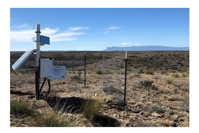
A TexNet seismic monitoring station. Hundreds of these stations are constantly monitoring seismic activity across Texas. Credit: Bureau of Economic Geology / The University of Texas at Austin
