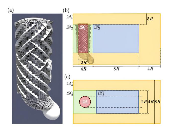
(a) Computational model for the study of passive ventilation in E. aspergillum.
