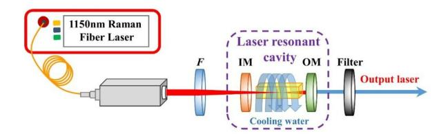
Schematic diagram of the experimental setup for end-pumped Ho,Pr:YAP crystal by 1150nm Raman laser. Credit: Zhang Huili
